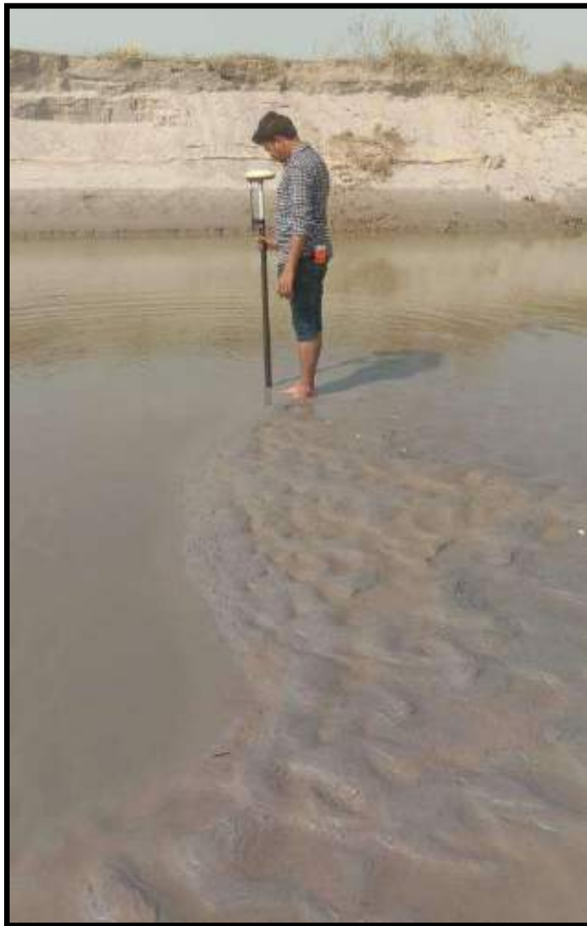
PHOTOGRAPH 5: DGPS survey for potential sand zone on Sutlej River, Ferozepur.
